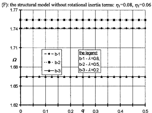
FIG. 6. Higher free vibration frequencies for the plate with concentrated masses ( $\eta = 50$ ).
