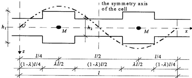
FIG. 7. The unit cell  $\Delta_1$  and the microshape function  $g$ .
