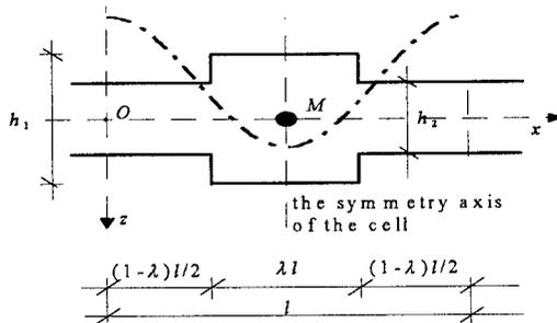
FIG. 2. The unit cell  $\Delta_1$  and the microshape function  $g$ .
