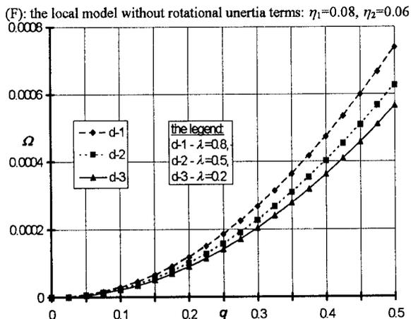
FIG. 5. Lower free vibration frequencies for the plate with concentrated masses ( $\eta = 50$ ).
