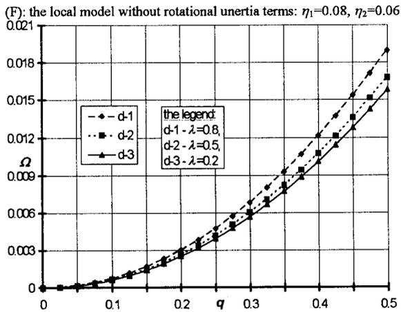
FIG. 3. Lower free vibration frequencies for the plate without concentrated masses ( $\eta = 0$ ).
