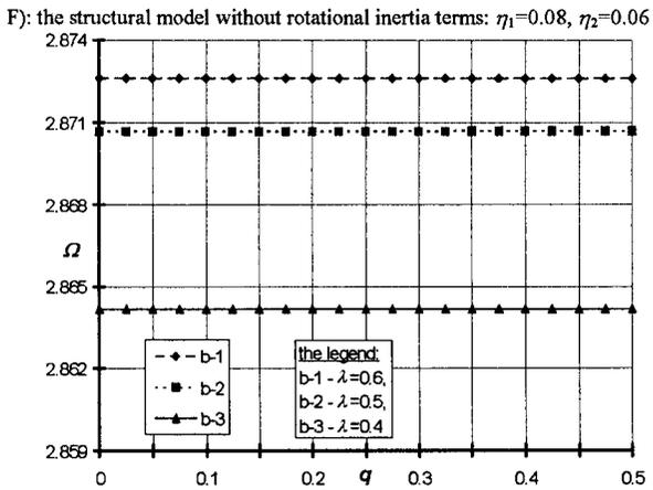
FIG. 4. Higher free vibration frequencies for the plate without concentrated masses ( $\eta = 0$ ).
