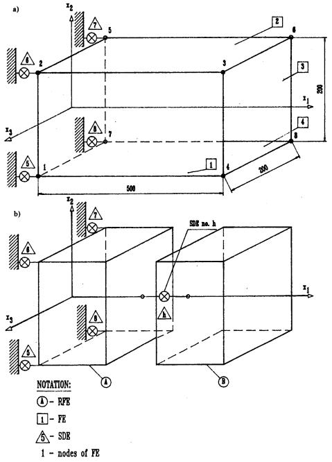
FIG. 11. The box frame: a) primary model, which is composed of FEs and SDEs, b) substitutive model, which contains the couple of two RFEs.
