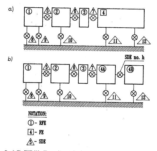
FIG. 8. The FWD 32J milling machine spindle: a) primary model, which is composed of RFEs and SDEs only, b) substitutive model, which contains the couple of new RFEs.
