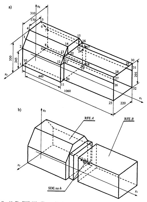
FIG. 12. The FWD 32J milling machine's beam: a) primary model, which is composed of FEs,b) substitutive model, which contains the couple of two RFEs.
