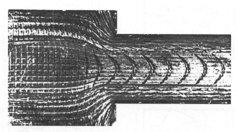
FIG. 5. Experimental grid distortion for Pb/OT3 composite (the hard core).
