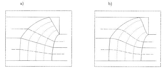
FIG. 3. Plastic zone and flow lines for both different models for Pb/OT3 composite (the hard core)  $\lambda = 3$  and  $R_0/R_c = 2$ .
