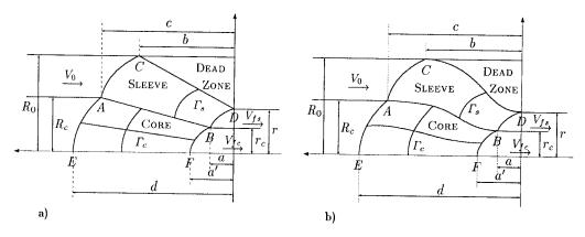
FIG. 1. General concept of the flow field construction in extrusion of bimaterial system: flow lines are straight a) or smooth b).
