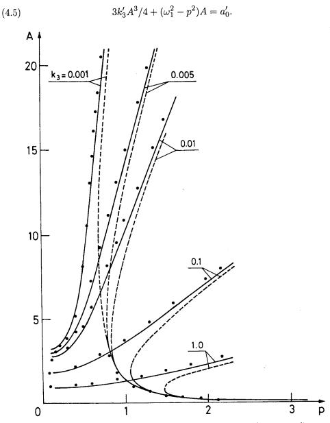
FIG. 2. Amplitude frequency curves according to Duffing's equation (continuous lines and dashed lines) and according to the wave approach in x = 0 (dotted lines) neglecting damping.
