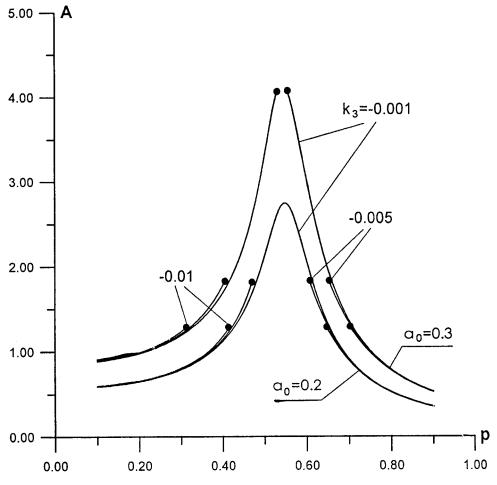
FIG. 8. Amplitude-frequency curves for  $k_3 = -0.001, -0.005, -0.01$  and  $a_0 = 0.2, 0.3$ .
