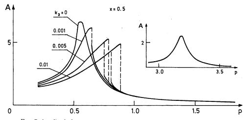
FIG. 7. Amplitude-frequency curves for x = 0.5 and  $k_3 = 0, 0.001, 0.005, 0.01$ .
