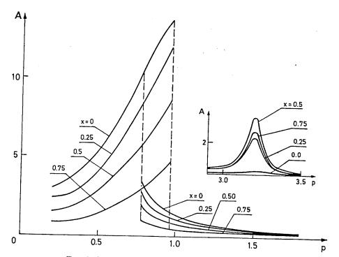
FIG. 3. Amplitude-frequency curves for  $d_0 = D_0 = 0.05$ .
