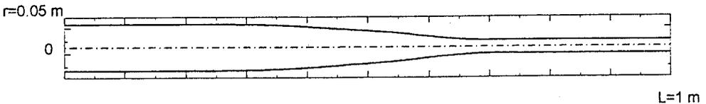
FIG. 4. Results of monocriterion optimization of the beam with respect to the maximum of  $\mu^*$ . The nondimensional area  $A$  of cross-section of the beam versus the nondimensional coordinate  $x$  and the shape of the cantilever beam for  $\beta_0 = 0$ .
