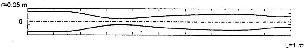
FIG. 8. Results of multicriterial optimization of the beam with respect to the maximum of  $\mu^*$ . The nondimensional area  $A$  of cross-section of the beam versus the nondimensional coordinate  $x$  and the shape of simply supported-fixed beam for  $\beta_0 = 0$ .
