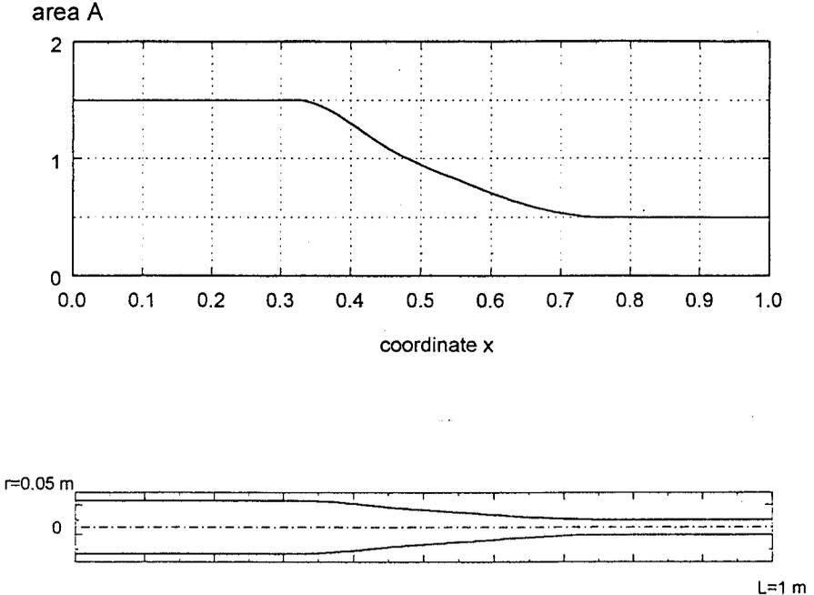
FIG. 6. Results of monocriterion optimization of the beam with respect to the maximum of  $\mu^*$ . The nondimensional area  $A$  of cross-section of the beam versus the nondimensional coordinate  $x$  and the shape of the cantilever beam for  $\beta_0 = 0.6$ .
