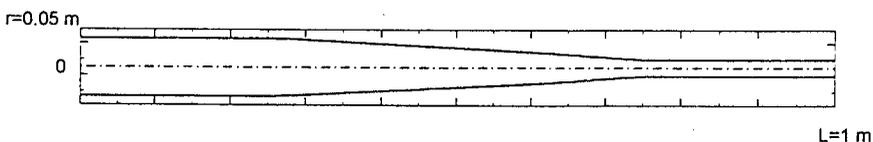
FIG. 5. Results of monocriterion optimization of the beam with respect to the maximum of  $\mu^*$ . The nondimensional area  $A$  of cross-section of the beam versus the nondimensional coordinate  $x$  and the shape of the cantilever beam for  $\beta_0 = 0.2$ .
