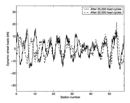
FIG. 5. Dynamic wheel forces from multi-leaf steel suspension on the outer wheel path.
