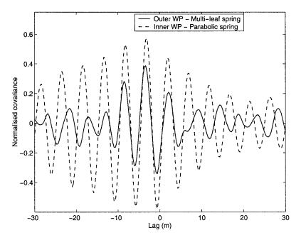
FIG. 10. Cross-covariance between wheel force and VSD for first test.
