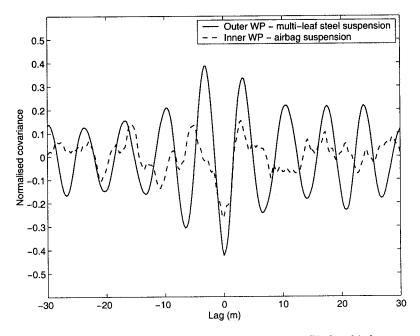
FIG. 15. Cross-covariance between wheel force and VSD for third test.
