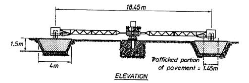
FIG. 1. Elevation view of CAPTIF.
