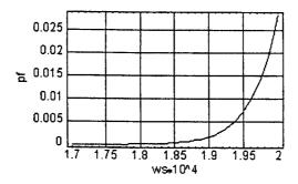
Fig. 4. The probability of failure calculated for the serviceability limit state vs. the expected value of the displacement.
