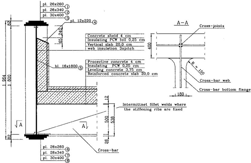
FIG. 5. Cross-section of the bridge.
