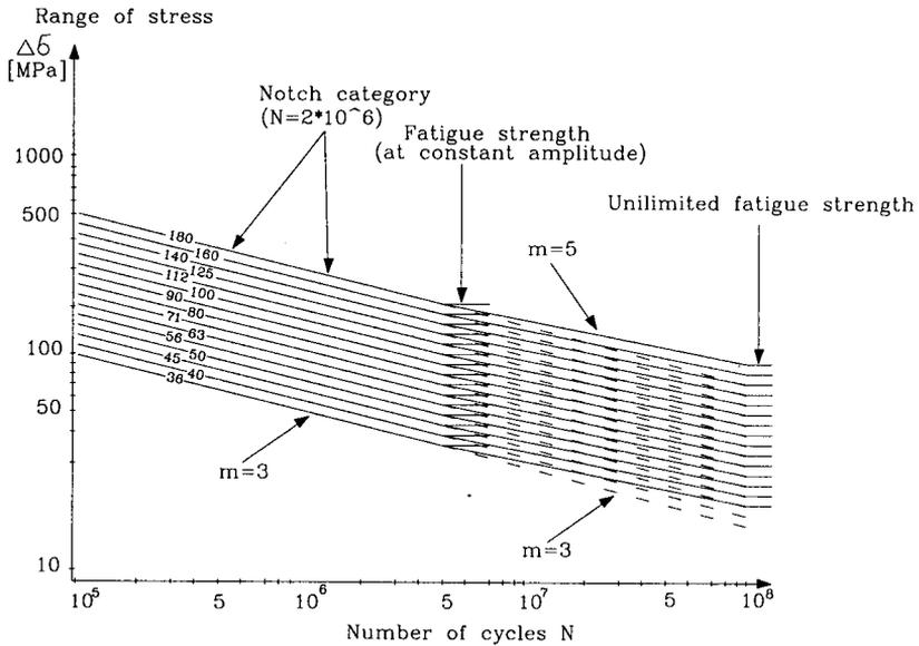
FIG. 1. Fatigue load capacity curve for different categories of notches.
