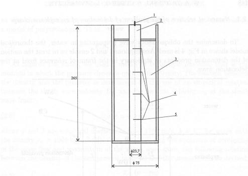
FIG. 2. System used in a water test: 1 - fuse, 2 - explosive charge, 3 - water, 4 - short-circuit sensors for measurement of detonation velocity, 5 - sensor releasing X-ray apparatus.
