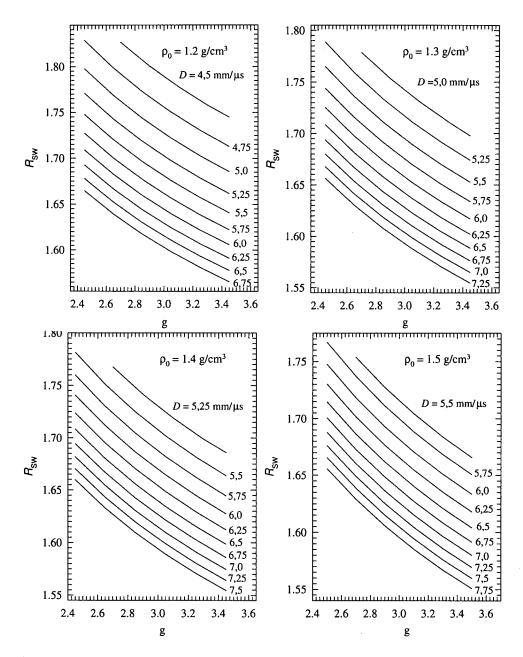
FIG. 5a Dependence of the dimensionless radial position of a shock wave in water,  $R_{SW}$ , calculated for an axial co-ordinate  $X_{SW} = 1$ , on the isentropic exponent of detonation products,  $\gamma$ .
