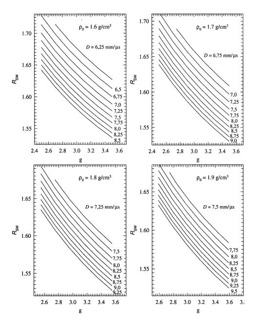
FIG. 5b Dependence of the dimensionless radial position of a shock wave in water,  $R_{SW}$ , calculated for an axial co-ordinate  $X_{SW} = 1$ , on the isentropic exponent of detonation products,  $\gamma$ .
