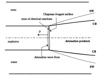
FIG. 1. Schematic image of detonation of a cylindrical explosive charge in a water envelope.
