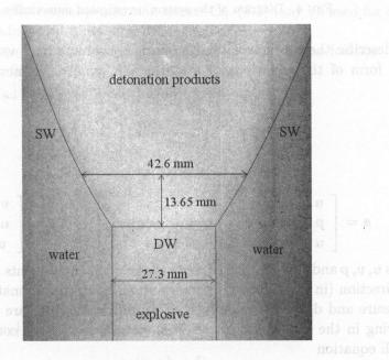
FIG. 3. An exemplary X-ray photograph of the initial stage of acceleration of a cylindrical layer of water.
