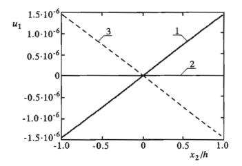
FIG. 2. Distribution of the displacement  $u_1$  over the thickness of a beam.
