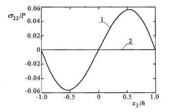
FIG. 6. Distribution of the normal stress  $\sigma_{22}$  over the thickness of a beam.
