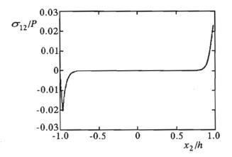
FIG. 7. Distribution of the tangential stresses  $\sigma_{12}$  over the middle surface.
