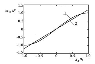
FIG. 4. Distribution of the normal stress  $\sigma_{11}$  over the thickness of a beam.
