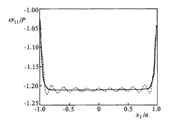
FIG. 10. Variation of the normal stress with the number of approximations.
