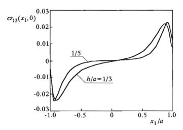
FIG. 9. Distribution of the tangential stress over the middle surface of a short beam.
