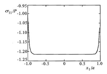
FIG. 5. Change of the normal stress  $\sigma_{11}$  on the lower surface of a beam.
