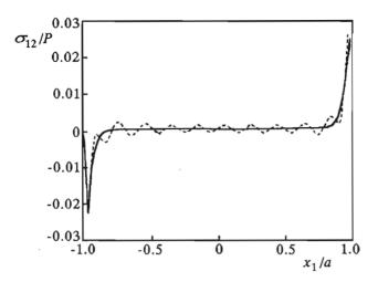
FIG. 11. Variation of the tangential stress with the number of approximations.
