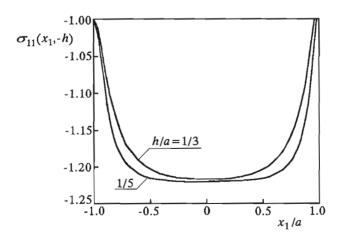
FIG. 8. Distribution of the normal stress over the bottom surface of a short beam.
