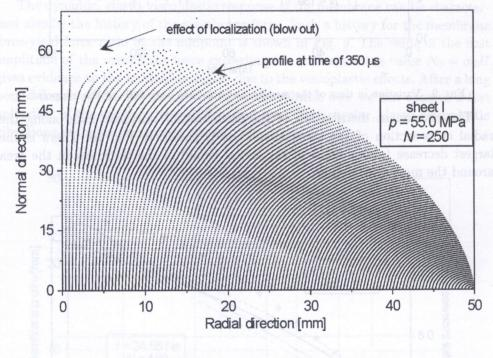
FIG. 11. Trajectories of the membrane particles.
