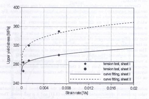
FIG. 2. Variation of the upper yield stress with strain rate for the mild steel specimen.
