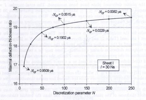
FIG. 4. Variation of the maximal deflection with the discretization parameter N as an illustration of the solution convergence.
