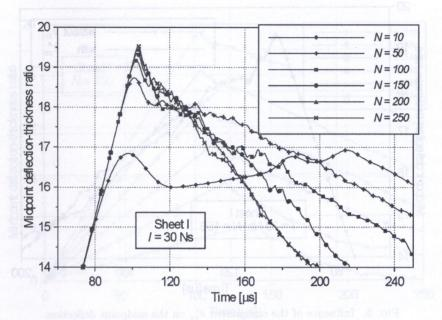
FIG. 3. Sensitivity of the membrane response to variation of the space discretization parameter N.
