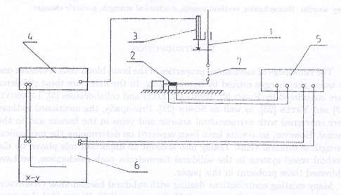
FIG. 1. Block diagram of the research stand: 1-microscarifier, 2-force sensor, 3-linear extension sensor, 4-mechanical quantities gauge, 5-stabilized electric feeder, 6-XY recorder, 7-test sample.
