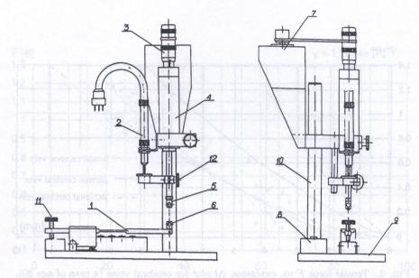
FIG. 2. Microscarifier: 1-force gauge beam, 2-linear extension sensor, 3-analog displacement indicator, 4-tightener unit, 5-upper mount seat, 6-lower mount seat, 7-actuator, 8-force gauge electrical unit, 9-base of microscarifier, 10-column, 11-preliminary tension correction screw, 12-preliminary tension control knob.
