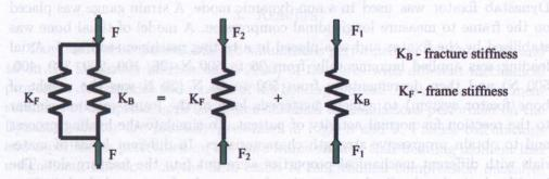
Fig. 5. Diagram of idealised fixator system as a two-spring system.
