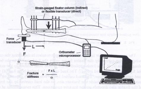
Fig. 2. Direct method of fracture stiffness measurement, after [3].
