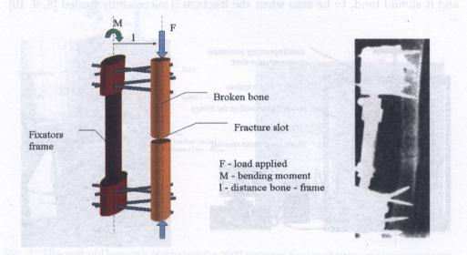
Fig. 4. Diagram of external fixator showing major components and applied loading with RTG photo.
