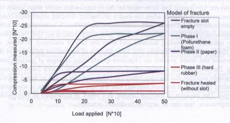
Fig. 10. Hysteresis loops of compression measured on the frame under the load applied for 5 models of fracture strength.
