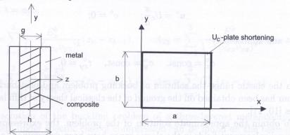
FIG. 2. Geometry and loading of a plate.
