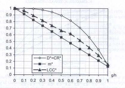
FIG. 6. Variation of dimensionless mass, critical stress and ultimate load for plates of a/h = 80 – steel faces (material parameters given in Fig. 5).
