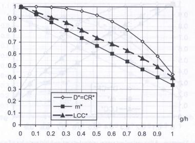
FIG. 8. Variation of dimensionless mass, critical stress and ultimate load for plates of a/h = 80 – aluminium faces (material parameters given in Fig. 7).
