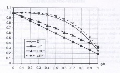
FIG. 4. Variation of dimensionless mass, critical stress and ultimate load for plates of a/h = 100 (material parameters given in Fig. 3).
