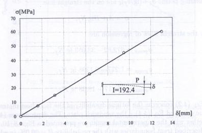
Fig. 6. The empirical dependence  $\sigma_g$  on  $\delta$  for the sandwich test pieces.
