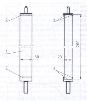
Fig. 2. The shape and dimensions of the test piece for fatigue investigations; 1 – polyvinyl chloride foam, 2 – lower holder, 3 – upper holder, 4 – adhesive layer.
