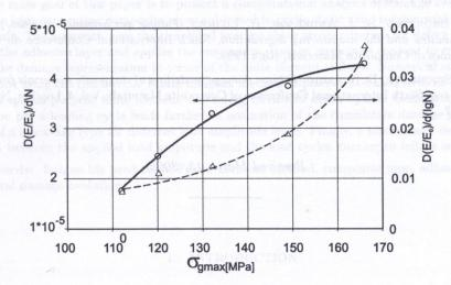
Fig. 14. The speed of changes of E modulus as a function of maximal stresses.
