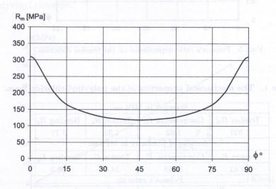
Fig. 3. Tensile strength dependence on the direction of the loading.
