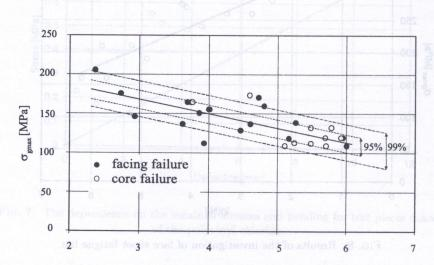
Fig. 10. Results of the investigation of sandwich structure for fatigue life in oscillatory bending.
