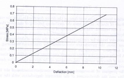
Fig. 7. The dependence on the maximal stresses and bending for test pieces made of the polyvinyl chloride.
