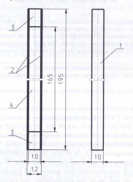
Fig. 1. The shape and dimensions of the test piece used in testing; 1 – test piece, 2 – face sheet, 3 – pads of aluminium alloy, 4 – core.
