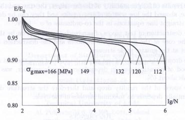
Fig. 13. The dependence of the relative drop of the elasticity modulus on the cycle number for the chosen maximal stresses.
