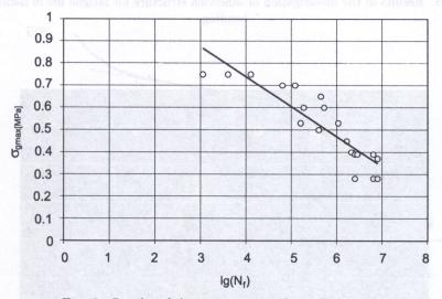
Fig. 9. Results of the investigation of core fatigue life.
