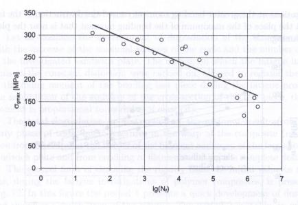
Fig. 8. Results of the investigation of face sheet fatigue life.
