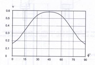
Fig. 5. Poisson's ratio dependence on the tension direction.
