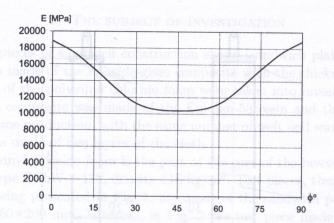
Fig. 4. The dependence of the elasticity of elongation modulus on the tension direction.
