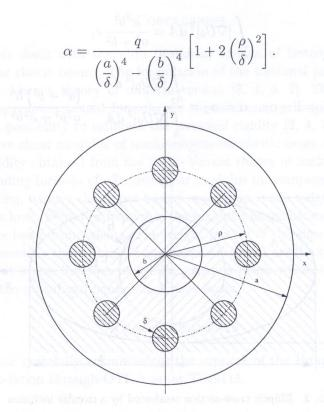
FIG. 1. Circular tube having a ring of circular inclusions.
