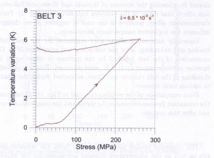
Fig. 14. Temperature changes vs. stress of woven polymer belt subjected to loading and unloading during tension test with the strain rate  $6.5 \times 10^{-3} \text{ s}^{-1}$ .
