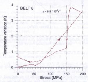
Fig. 16. Temperature changes vs. stress obtained during the relaxation test of woven polymer belt.
