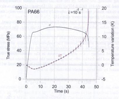
FIG. 6. Stress and temperature changes vs. time of solid polyamide PA66 sheet sample subjected to tension test with strain rate  $10^{-2}$  s<sup>-1</sup>.
