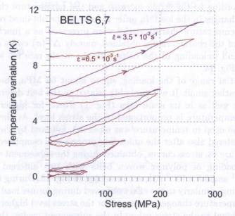
Fig. 15. Temperature changes vs. stress obtained for woven polymer belt during subsequent tension tests with strain rates  $6.5 \times 10^{-3} \text{ s}^{-1}$  and  $3.5 \times 10^{-2} \text{ s}^{-1}$ .
