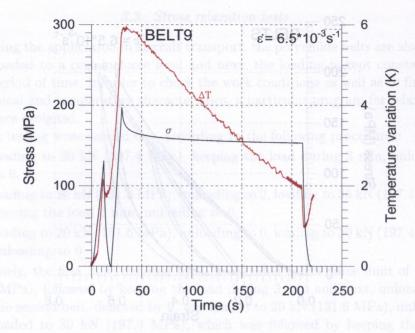
Fig. 12. Stress and temperature vs. time of woven polyamide belt subjected to loading, unloading and stress relaxation sequences in the second cycle of loading.
