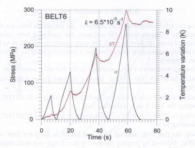
Fig. 9. Stress and temperature curves of polyamide woven belt subjected to subsequent cyclic test with strain rate  $6.5 \times 10^{-3}$  s<sup>-1</sup>.
