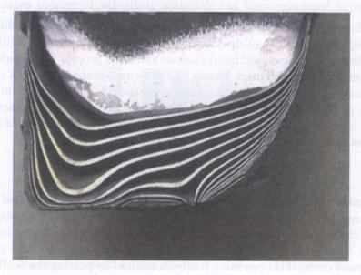
FIG. 2. Deformed layers of aluminium alloy (dual – channel extrusion).
