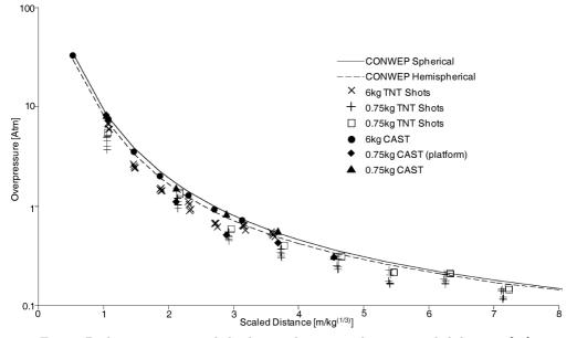
FIG. 2. Peak overpressure and shock arrival time in relation to scaled distance [16].
