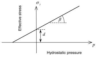
FIG. 4. Linear Drucker-Prager model in meridional plane.
