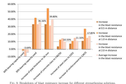
FIG. 9. Breakdown of blast resistance increase for different strengthening solutions.
