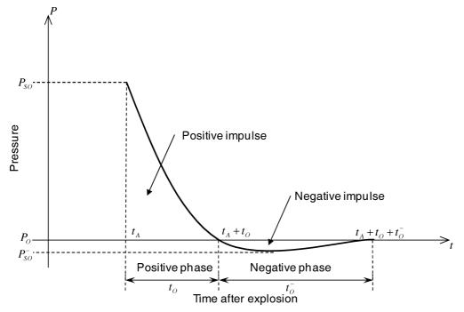
FIG. 1. Relation between time and shock wave pressure.
