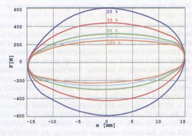
FIG. 8. Damping force as a function of piston displacement for various control openings of the servo-valve, vibrations frequency 3 Hz.
