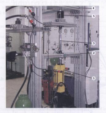
FIG. 1. Experimental stand with a commercially available shock absorber mounted in between the platforms.
