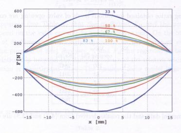
FIG. 13. Damping force vs. piston displacement for variable valve setting levels, at vibration frequency 3 Hz.
