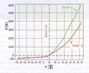
FIG. 3. Comparison of damping characteristics depending on the piston velocity for two oil temperatures.
