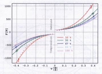
FIG. 12. Comparison of experimental characteristics and those derived from the nonlinear model.
