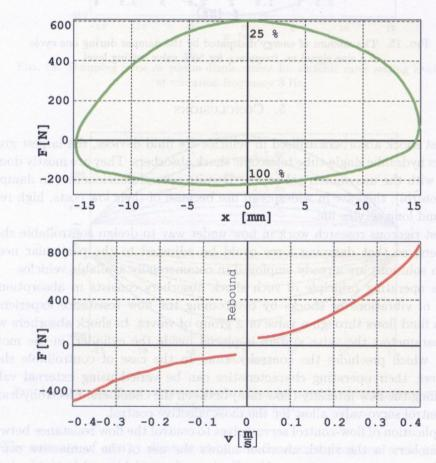
FIG. 16. Shaping the characteristics of a controllable servo-valve.
