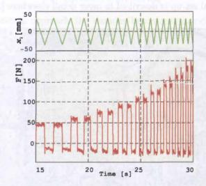
FIG. 2. Displacement and damping force in the function of time in the part of the experimental program.
