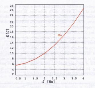
FIG. 15. The amount of energy dissipated by the damper during one cycle of a sine signal vs. frequency for 50% valve setting level.
