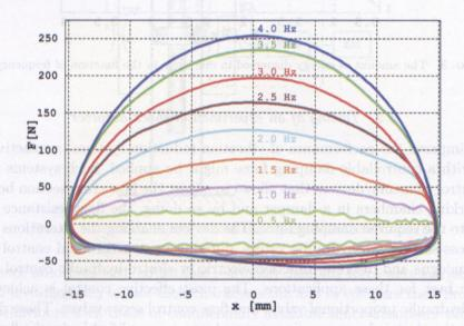
FIG. 4. Damping force as the function of piston displacement obtained by altering the vibrations frequency.
