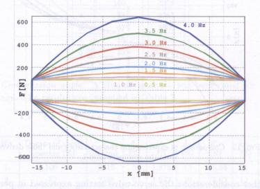
FIG. 14. Damping force vs. piston displacement for variable vibration frequency, at 50% valve setting level.
