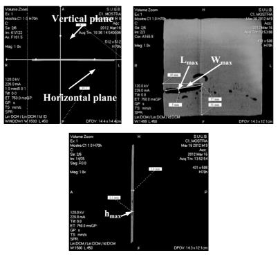
FIG. 3. Processing of the tomographic images.
