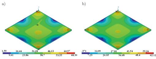
FIG. 11. Contour map of the non-dimensional von Mises equivalent stress: a) flawed plate, b) calibration plate.
