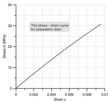
FIG. 9. The average stress-strain curve of the polyesteric resin.
