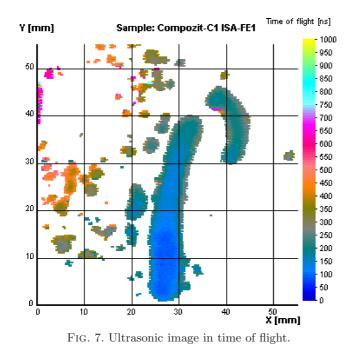
The image in amplitude was used to measure the position and dimensions of defects while the image in time of flight was used to obtain the depth of defects.
