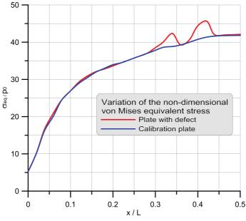
FIG. 12. Comparative variation of the von Mises equivalent stress in the middle section on line MN.
