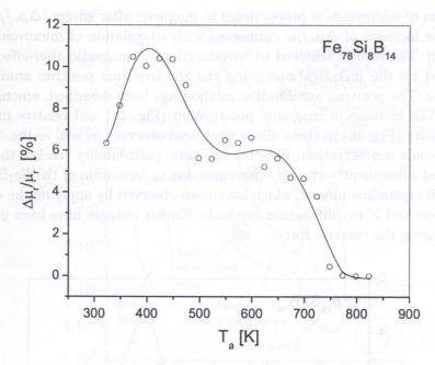
Fig. 12. Changes of magnetic after-effects  $\Delta \mu_r/\mu_r$  versus one-hour annealing temperature  $T_a$  for Fe<sub>78</sub>Si<sub>8</sub>B<sub>14</sub> alloy.
