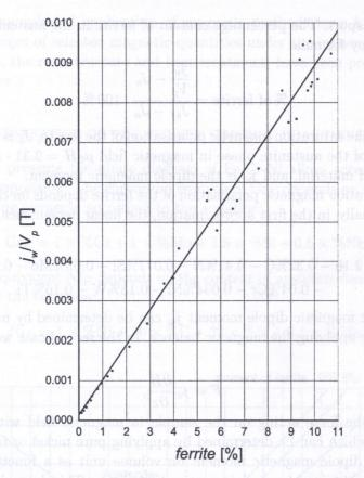
Fig. 2. Magnetic dipole moment on volume unit measured by applying magnetic balance as a function of ferrite concentration in the Fe-Cr-Ni alloys.
