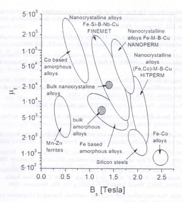
Fig. 15. The dependence of relative magnetic permeability  $\mu_r$  versus saturation magnetic induction  $B_s$  (f=1 kHz) for conventional and bulk amorphous alloys, conventional and bulk nanocrystalline alloys, and selected crystalline alloys [10, 24–26].
