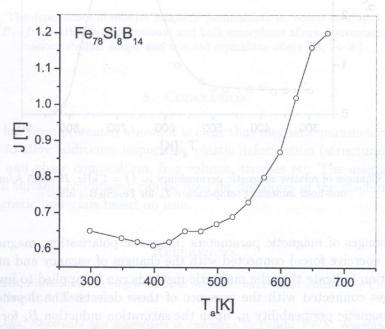
Fig. 13. Changes of magnetic polarisation versus one-hour annealing temperature  $T_a$  for Fe<sub>78</sub>Si<sub>8</sub>B<sub>14</sub> alloy.
