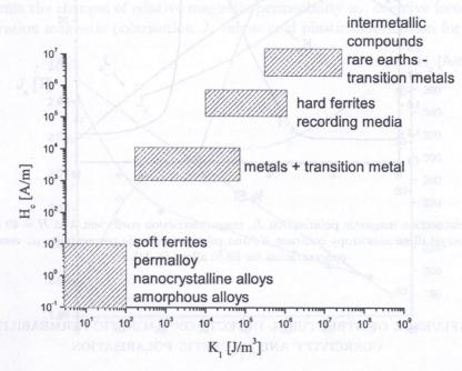
Fig. 6. Coercivity  $H_c$  of soft and hard magnetic materials as a function of the magnetocrystalline anisotropy constant  $K_1$  [16].
