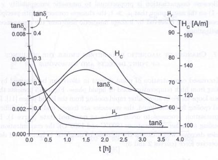
Fig. 11. Changes of coercivity  $H_c$ , relative magnetic permeability  $\mu_r$ , tangent of magnetic hysteresis losses  $\tan \delta_h$ , and relaxation magnetic losses  $\tan \delta_r$  during ageing at the temperature 523 K after supersaturation from the temperature 973 K to 273 K in  $\alpha$ Fe - 0.02%C [20].
