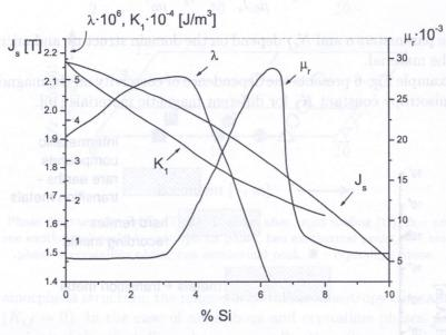
Fig. 7. Saturation magnetic polarisation  $J_s$ , magnetostriction coefficient  $\lambda$  at H=40 A/cm, magnetocrystalline anisotropy constant  $K_1$  and relative magnetic permeability  $\mu_r$  versus Si concentration for Fe-Si alloys [8, 11].
