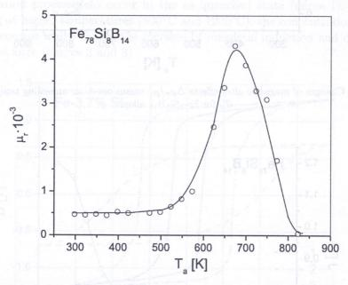
Fig. 14. Changes of relative magnetic permeability  $\mu_r$  (f=1 kHz, H=0.5 A/m versus one-hour annealing temperature  $T_a$  for Fe<sub>78</sub>Si<sub>8</sub>B<sub>14</sub> alloy.
