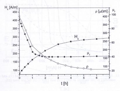
Fig. 12. Coercivity  $H_c$ , relative magnetic permeability  $\mu_r$ , and resistivity  $\rho$  measured at room temperature versus aging time t at the temperature 423 K after supersaturation from 863 K to 273 K in  $\alpha$ Fe - 0.012%N [20].
