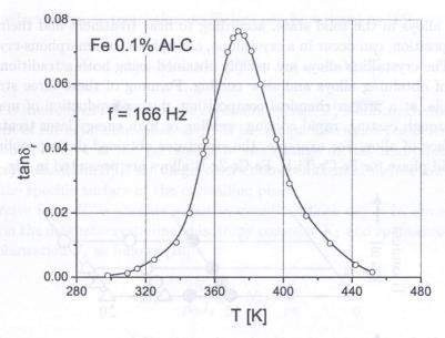
Fig. 4. Tangent of relaxation losses as a function of temperature in Fe containing 0.1% Al-0.007% C.
