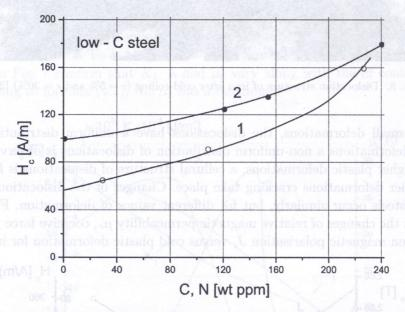
Fig. 10. Coercivity as a function of C and N concentration in high-purity steel; (1) after ageing treatment, (2) before ageing treatment [11].
