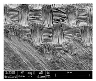
FIG. 4. Boundary between a worn original surface and fibers for PMCs.
