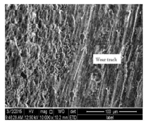
FIG. 5. SEM micrograph of the worn surface of NiCr coating.
