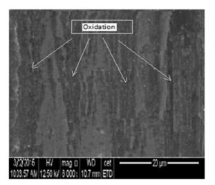
FIG. 6. Formation of oxide films on the worn surface of NiCr at high temperature (300°C).
