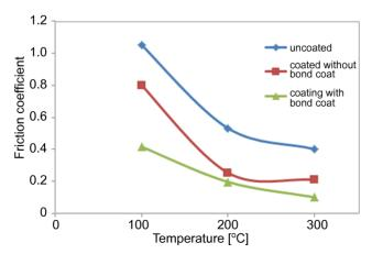
FIG. 2. Friction coefficient of coated and uncoated PMCs as a function of temperature.
