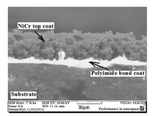
FIG. 8. SEM images of cross-section of PMCs with polyimide bond coating layer and NiCr top coating layer.
