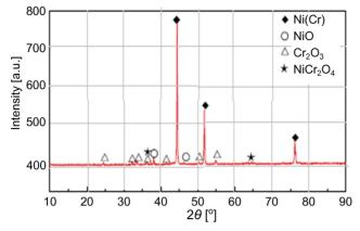
FIG. 7. XRD patterns of worn surface of NiCr at 300°C.
