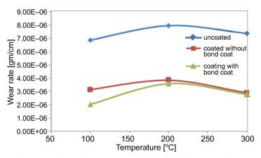
FIG. 1. Wear rate of coated and uncoated PMCs as a function of temperature.
