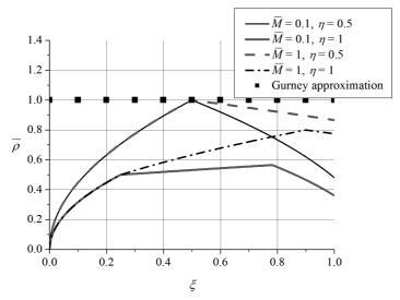
FIG. 5. Variation of the relative density,  $\overline{\rho}$ , of the DPs versus Lagrangian coordinate,  $\xi$ , for selected values of  $\eta$  and  $\overline{M}$ .
