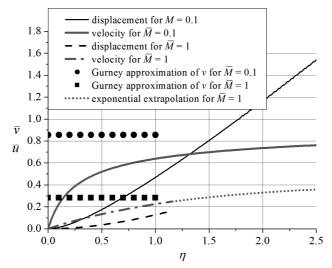
FIG. 6. Variation of the relative displacement and velocity of metal plate versus relative time  $\eta$ , for selected values of  $\overline{M}$ .
