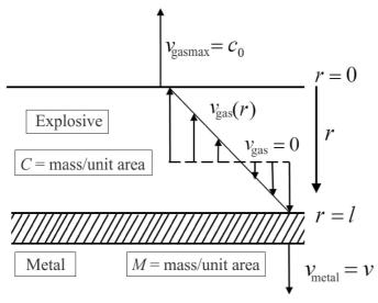
FIG. 2. The linear profile of DPs velocity versus Lagrangian coordinate, r, for an OFS.
