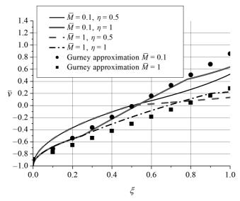
FIG. 4. Variations of the relative velocity,  $\overline{v}$ , of the DPs versus Lagrangian coordinate,  $\xi$ , for selected values of  $\eta$  and  $\overline{M}$  (on the background linear Gurney approximation).
