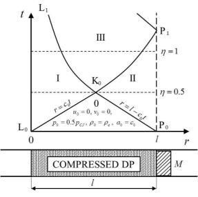
FIG. 3. Part of the network of limiting characteristics in the space between piston and free surface.
