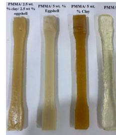
FIG. A2. Fabricated specimens of pure PMMA and its composites.
