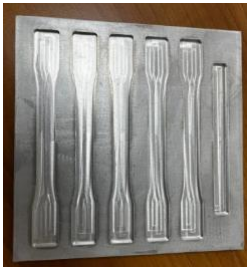
FIG. A1. Tensile mold made of aluminum.
