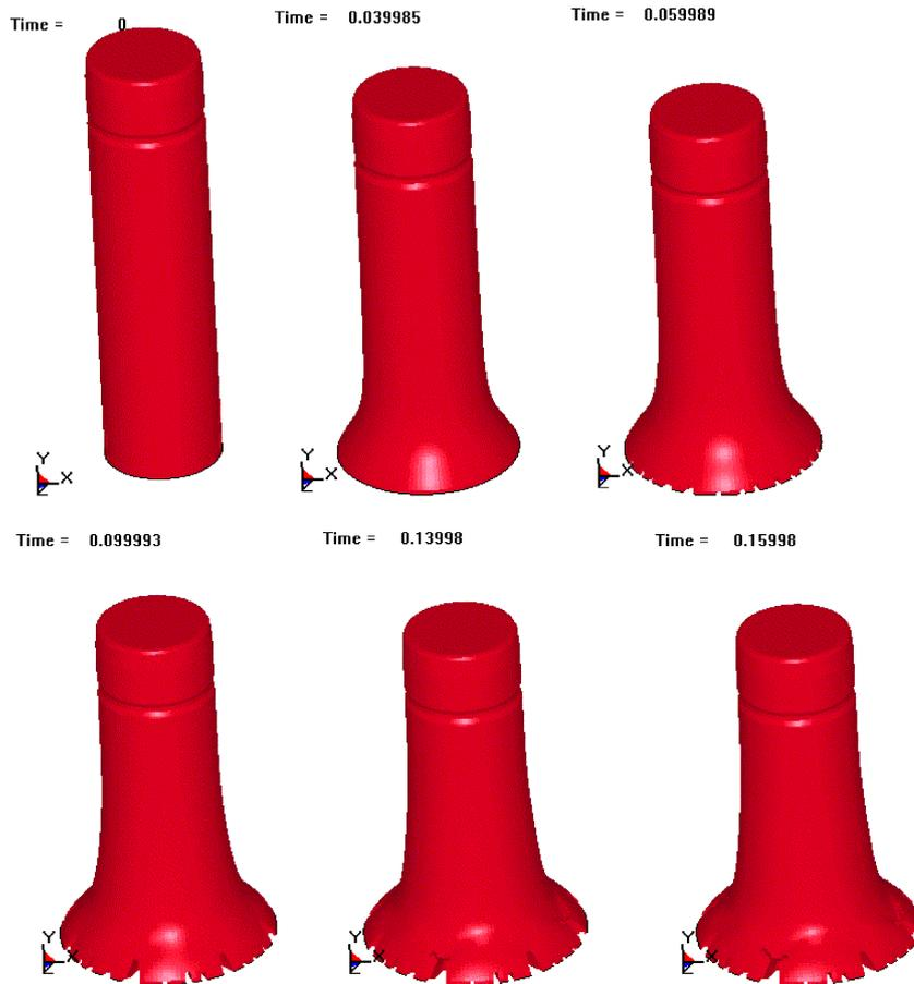
FIG. 16. Deformation failure process of 45 steel Taylor impact specimen (310 m/s).
