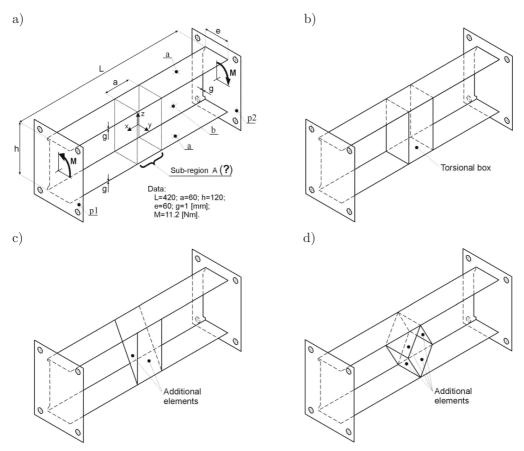
FIG. 1. Formulation of design problem for a thin-walled channel beam loaded with torsion moment and selected solutions analysed with FEM.
