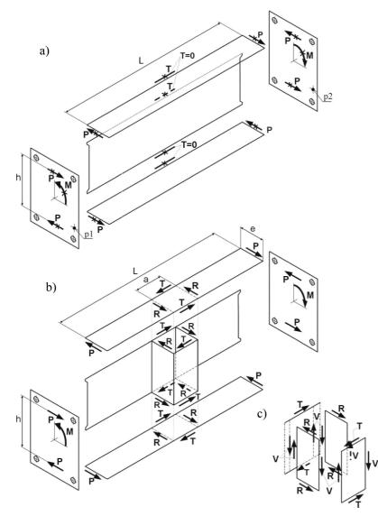
FIG. 6. Statical analyses for regular thin-walled channel beam and the beam reinforced with torsional box [2].
