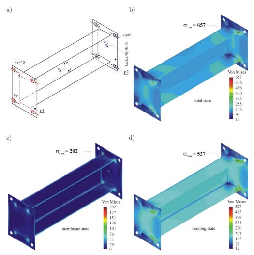
FIG. 2. Constructional scheme of model of regular thin-walled channel beam, boundary conditions assumed for FEM calculations and distributions of equivalent stresses calculated according to Huber-Misses criterion.
