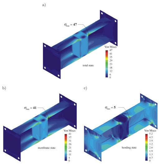
FIG. 3. Results of FEM analyses for the model of thin-walled channel beam reinforced with a torsional box.
