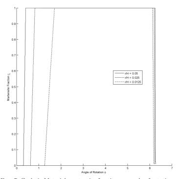
FIG. 7. Cycle 1: Material martensite fraction vs. angle of rotation  $\phi.$
