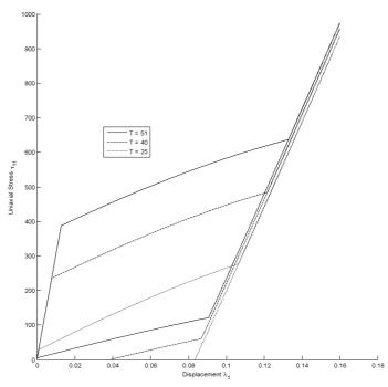
FIG. 2. Uniaxial tension. Uniaxial stress  $\tau_{11}$  vs. axial strain  $\lambda_1$  for different values of the (reference) temperature T.
