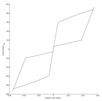
FIG. 3. Torsion of an SMA tube: Shear stress  $\tau_{\theta z}$  vs. relative angle of twist  $\phi$ .
