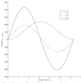
FIG. 9. Cycle 2 (r/H=0.05): Stresses vs. angle of rotation  $\phi.$
