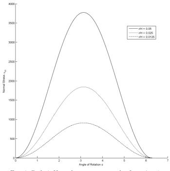
FIG. 4. Cycle 1: Normal stress  $\tau_{11}$  vs. angle of rotation  $\phi.$
