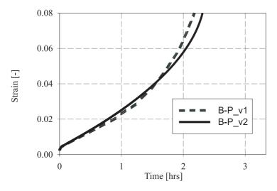
Fig. 5. Creep curves for B1900+Hf at 982° C,  $\sigma = 283$  [MPa] = const.
