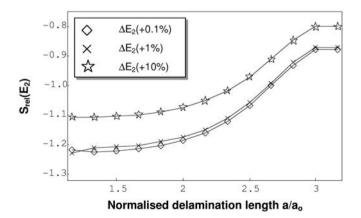
FIG. 13. Relative sensitivities of the fracture parameter with respect to the Young's modulus  $E_2$  – forward finite difference.
