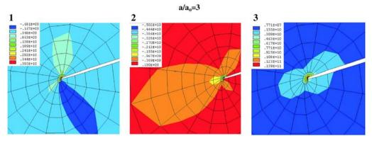
FIG. 12. Near-crack tip stress distribution  $(+\Delta E_2 = 10\%)$  [Pa] (1) normal (2) shear (3) von Mises.
