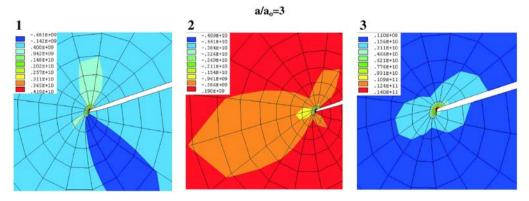
FIG. 11. Near-tip stress distribution for nominal design parameter values [Pa] (1) normal (2) shear (3) von Mises.
