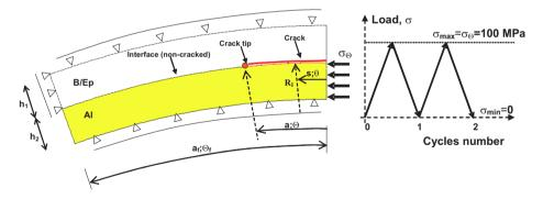
FIG. 4. Two-layer boron/epoxy-aluminium curved composite under cyclic shear.
