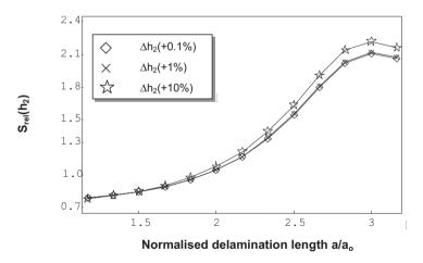
FIG. 7. Relative sensitivities of the fracture parameter with respect to the layer thickness  $h_2$ .
