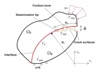
FIG. 1. Two-component model of a delaminated composite laminate.
