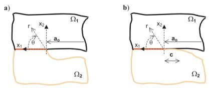
FIG. 2. Near-tip behaviour during fatigue delamination a) opened crack tip b) closed crack tip.
