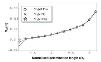
FIG. 8. Relative sensitivities of the fracture parameter with respect to the interface radius  $R_I$ .
