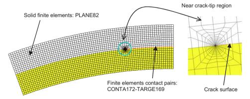
FIG. 5. FEM discretisation of composite domain and crack surfaces.
