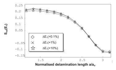
FIG. 6. Relative sensitivities of the fracture parameter with respect to the Young's modulus  $E_1$ .
