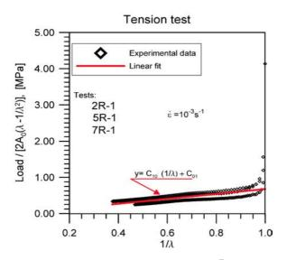
Fig. 1. Dependence of the change of reduced stress  $\frac{P}{2A_0 - \lambda - \frac{1}{\lambda^2}}$  as a function of the
