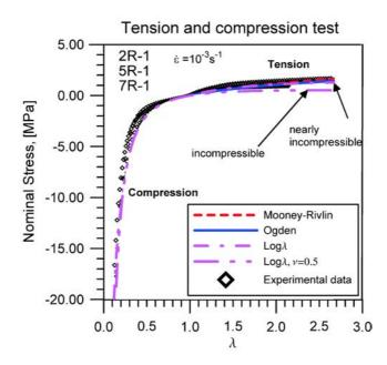
Fig. 4. The nominal stress in uniaxial tension and compression tests as a function of the axial stretch  $\lambda$ , for different constitutive models, Eqs. (3.6), (3.8), (3.12) (broken and solid lines). Experimental data (diamond marks) from Kwiecień *et al.* [20, 21].
