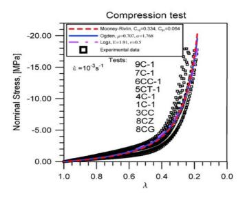
Fig. 3. The nominal stress as a function of the axial stretch  $\lambda$  for polyurethane rubber, in uniaxial compression test with strain rate  $3 \times 10^{-3} \text{ s}^{-1}$  for different constitutive models relations Eqs. (3.6), (3.8), (3.12) (broken and solid lines). Experimental data (quadrate marks) from Kwiecień *et al.* [20, 21].
