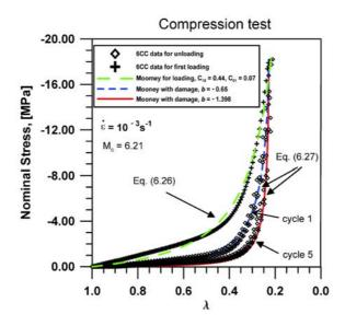
Fig. 7. Nominal stress in uniaxial cycle compression tests as a function of axial change of length  $\lambda$  for loading test (experimental data) and relation Eq. (6.26), and two extreme paths of unloading from the states with maximum intensities of strain M defined for identified models with damaged microstructure described by Eq. (6.27).
