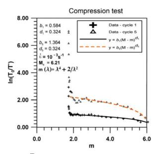
Fig. 10. The value of  $\ln \frac{T_{0 \ 11}}{T_{11}^*} = \ln \frac{\sigma_{11}}{\sigma_{11}^*}$  in uniaxial compression test as a function of strain intensity m for unloading test (experimental data), with two identified forms of function  $\xi = e^{-b(M-m)^d}$  for extreme cycles of unloading.
