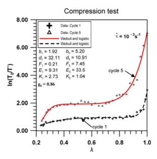
Fig. 11. The value of nominal stress in uniaxial cycle compression tests as a function of axial change of length  $\lambda$  for loading test (experimental data) and two extreme paths of unloading from the states with maximum intensities of strain M defined for identified models with damaged microstructure described by Eqs. (6.21) and (6.22),  $\xi^*(\lambda) = K(1 - g(\lambda))e^{-b(\lambda)^d}$ .
