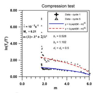
FIG. 9. The value of  $\ln \frac{T_{0 \ 11}}{T_{11}^*} = \ln \frac{\sigma_{11}}{\sigma_{11}^*}$  in a uniaxial compression test as a function of strain intensity m for unloading test (experimental data), with two identified forms of function  $\xi = e^{-b(m-\sqrt{3})^d}$  for extreme cycles of unloading.
