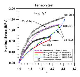
Fig. 5. Nominal stress in uniaxial tension test as a function of axial change of length  $\lambda$  for loading test (experimental data) and relation Eq. (6.24), and three expected paths of unloading from the states with maximum intensities of strain M, defined just before rupture  $\lambda = \lambda_{\text{max}}$ , for different samples described by Eq. (6.25) with the same damage parameter b.
