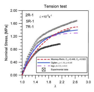
Fig. 2. The nominal stress as a function of the axial stretch  $\lambda$  for polyurethane rubber in a uniaxial tension test, with strain rate  $3 \times 10^{-4} \, \mathrm{s}^{-1}$  for different constitutive models relations Eqs. (3.6), (3.8), (3.12) (broken and solid lines). Experimental data (quadrate marks) from Kwiecień *et al.* [20, 21].
