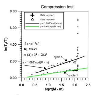
FIG. 8. The value of  $\ln \frac{T_{0 \ 11}}{T_{11}^*} = \ln \frac{\sigma_{11}}{\sigma_{11}^*}$  in uniaxial compression test as a function of  $\sqrt{M-m}$  for unloading test (experimental data) and two extreme values of identified damage parameter b (for first cycle b=0.48 and for last cycle b=1.093) with M=1.2 for one sample.
