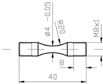
FIG. 1. Design of the specimen. Dimensions in mm.
