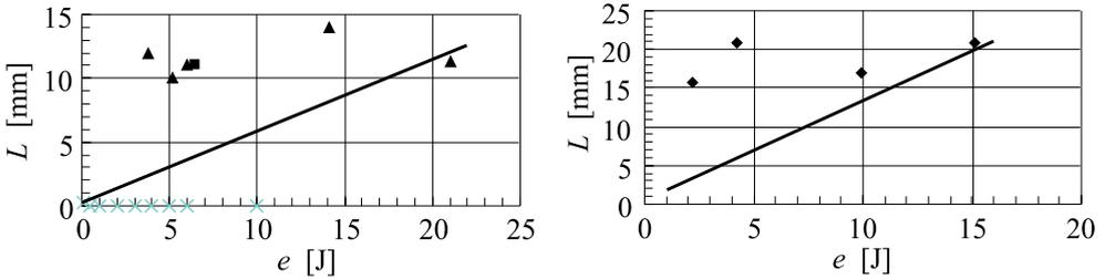
FIG. 4. Dependence of the penetration depth  $L$  on the impact energy  $e$  of needles No. 10 for steel and duralumin as targets (on the left) and of needles No. 7 and 10 for aluminum as a target (on the right). The meaning of symbols is as in Fig. 3. Solid lines denote calculations for plastic work at  $P_1^* = 2.5$  and  $0.86$  GPa for duralumin and aluminum respectively.
