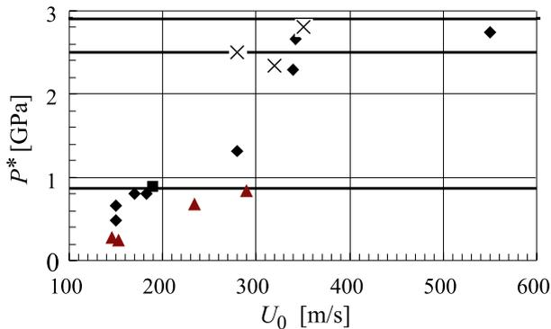
FIG. 3. Dependence of the resistance  $P^*$  to penetration of needles on the impact velocity  $U_0$ .
