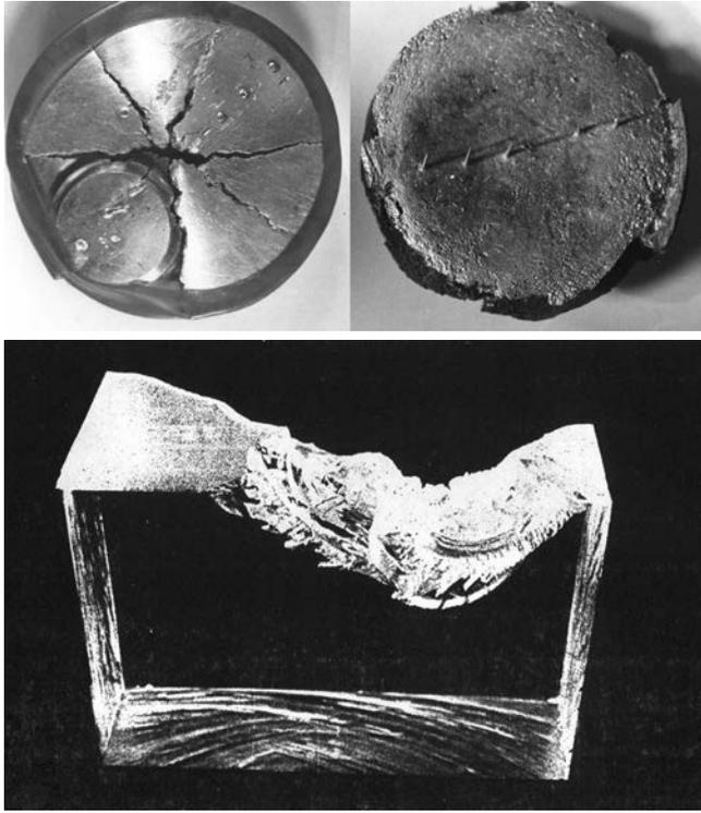
FIG. 2. Results of the impact of needles on the targets of duralumin, steel, and plexiglas.
