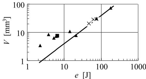
FIG. 5. Dependence of the channel volume  $V$  on the needle energy  $e$  for different materials. The meaning of symbols is as in Fig. 3. The curve denotes the calculations for plastic work at  $P_1^* = 2.5$  GPa for duralumin.
