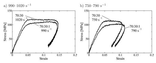
FIG. 7. Effect of dialkylperoxide addition on stress-strain curve for PLA:PBAT = 70:30 and PLA:PBAT:dialkylperoxide = 70:30:1.
