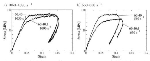
FIG. 6. Effect of dialkylperoxide addition on the stress-strain curve for PLA:PBAT = 60:40 and PLA:PBAT:dialkylperoxide = 60:40:1.
