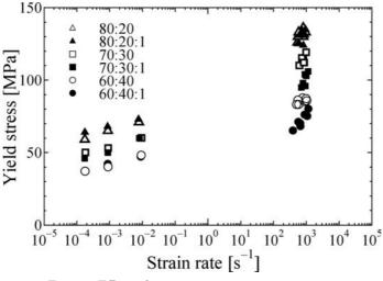
FIG. 8. Effect of strain rate on maximum stress.
