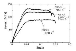
FIG. 5. Effect of PBAT content on stress–strain curves at strain rates of  $960-1050 \text{ s}^{-1}$ .
