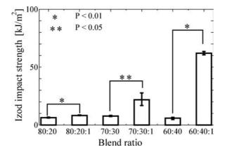
FIG. 4. Impact resistance of different PLA/PBAT alloys.
