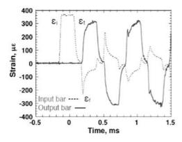
FIG. 5. Measured strain data.
