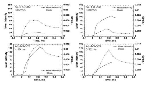
FIG. 6. Comparison of the strain and luminescence as a function of time.
