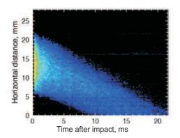
FIG. 4. Luminescence distribution along the central horizontal line.
