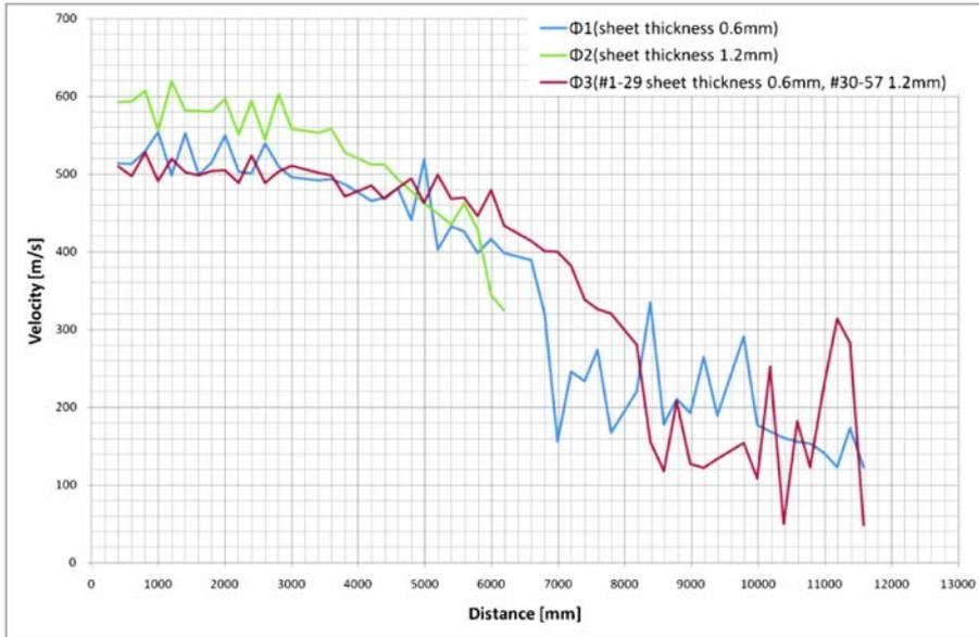
FIG. 15. Distance-velocity data using 155 mm smooth bore gun.
