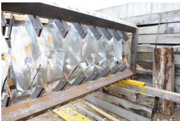
FIG. 11. Deformed plates end section.
