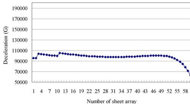
FIG. 2. Estimation of thickness distribution of plate array for soft recovery of projectile: a) thickness distribution of sheet array, b) estimated deceleration of a projectile.
