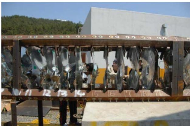
FIG. 10. Deformed plates, mid section.
