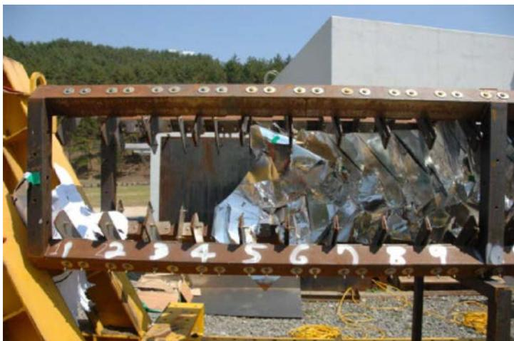
FIG. 9. Deformed plates, front section.
