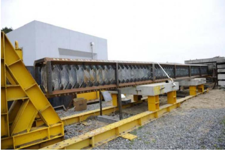
FIG. 3. Soft recovery system with plates installed.
