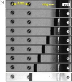
FIG. 5. The example of screen shot of graphical user interface presented video window with the moving ring segment and expansion velocity curve calculated with the use of TEMA Automotive software (a), and the sequence of images showing the observation area with the moving ring segment (b).
