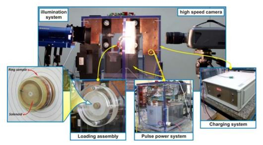
FIG. 4. View of the arrangement for electromagnetic ring experiment.
