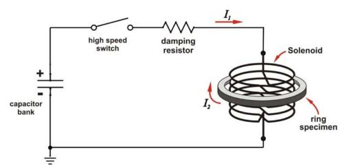
FIG. 3. Schematic diagram of the arrangement for electromagnetic ring expansion.
