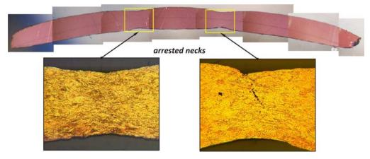
FIG. 7. View of the annealed copper ring fragment and the structures of the arrested necks arisen into ring fragment.
