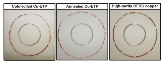
FIG. 6. View of recovered fragments generated from different sorts of copper rings.
