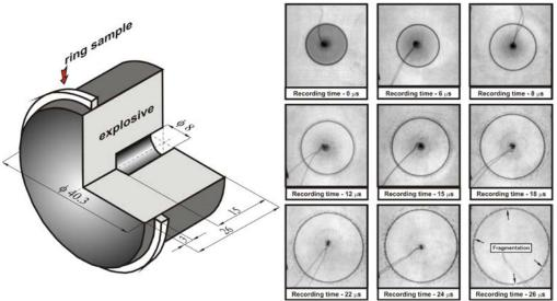
FIG. 2. Scheme of the experimental set-up driving explosively the ring sample (a) and radiographs of explosively expanding rings made of copper sinter (b) [9].
