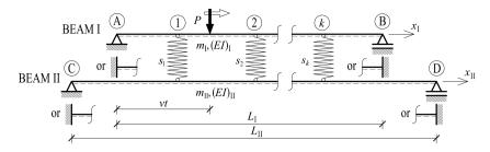
FIG. 1. Double-beam system with intermediate elastic restraints subjected to a moving force.
