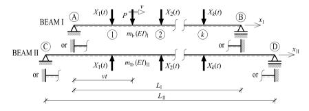
FIG. 2. Two single-span beams subjected to moving force and redundant forces.
