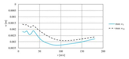
FIG. 8. Maximum dynamic deflection throughout the upper and the lower beam *versus* different force movement velocities.
