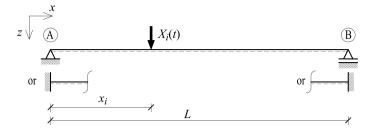
FIG. 4. Single-span beam subjected to a concentrated time-varying force.
